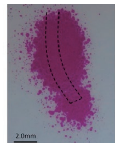
Analysis of cavitation of ultrasonically activated devices using pressure measurement film
